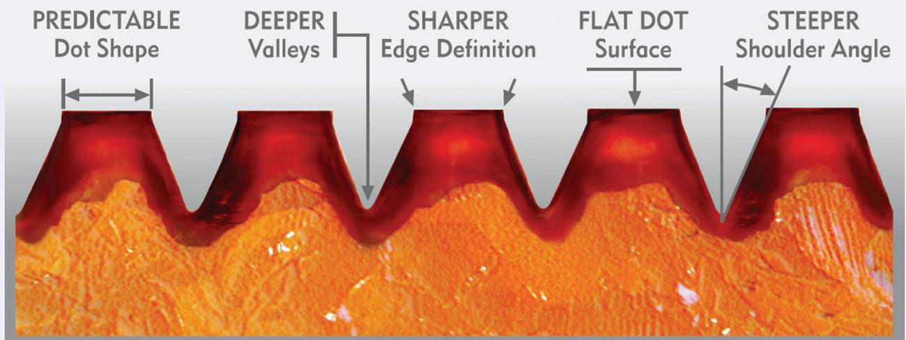
CSW found MacDermid’s LUX platemaking technology met its needs for flat-top dots, sharp edges, and steep shoulder to support its corrugated customers.
