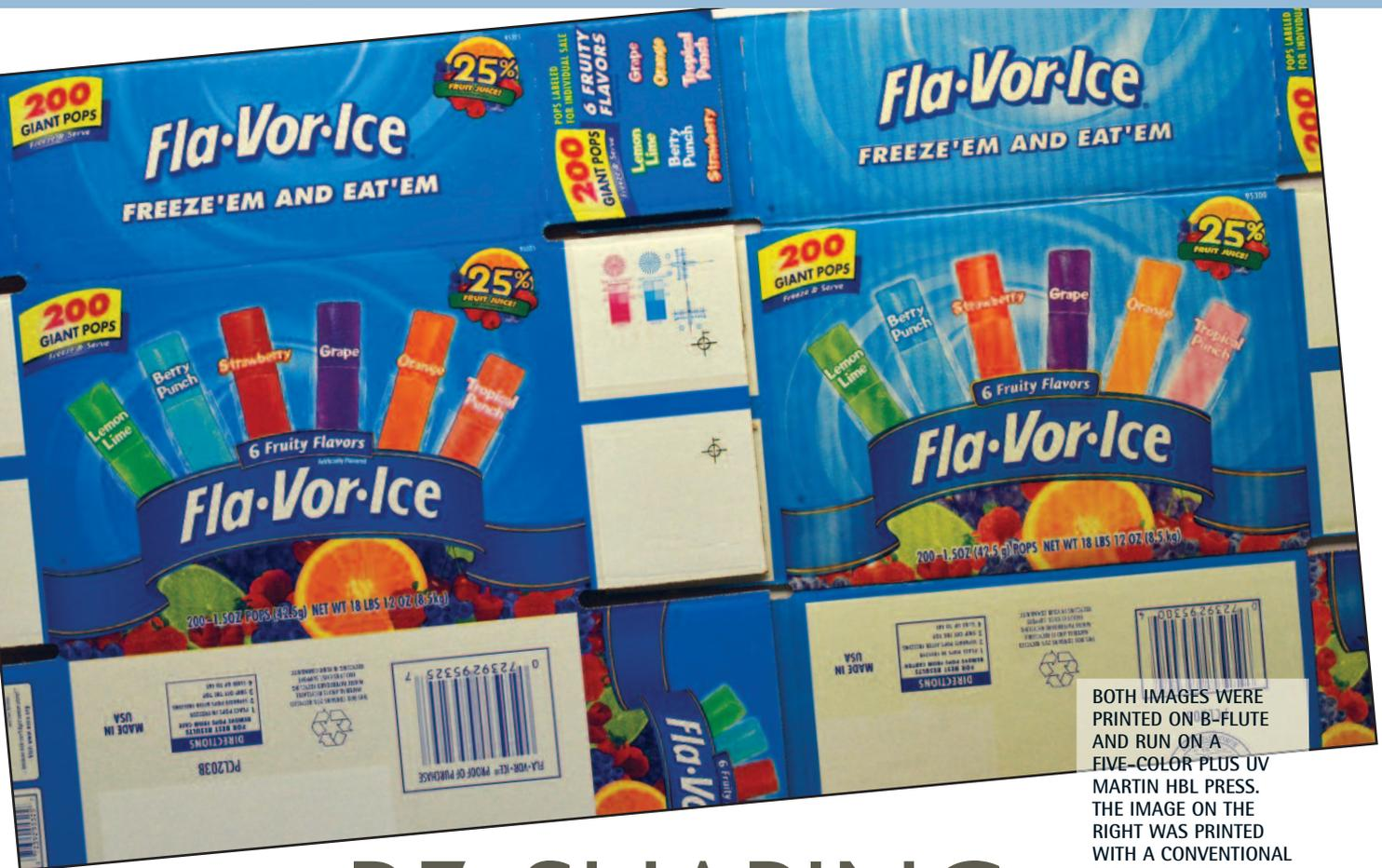
BOTH IMAGES WERE PRINTED ON B-FLUTE AND RUN ON A FIVE-COLOR PLUS UV MARTIN HBL PRESS. THE IMAGE ON THE RIGHT WAS PRINTED WITH A CONVENTIONAL DIGITAL PLATE. THE DESIGN ON THE LEFT WAS PRINTED WITH A LUX PRINTING PLATE.
